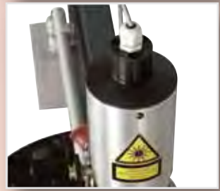
Cylinder prepared for installing a laser pointer
