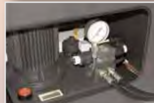
Two circuit hydraulic unit in cabinet base
