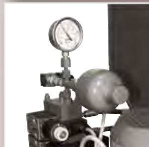
Two-circuit hydraulic unit
