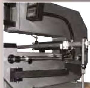
Length and depth stop on both sides in double spherical guides. 2 Adjustable stops on the right and left side of the Y-axis.
