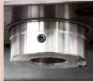
Stable piston rod ( \varnothing 55 mm) with anti-twist tool protection
