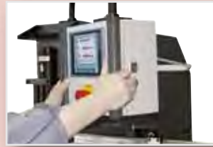
Control panel with two-hand operation
