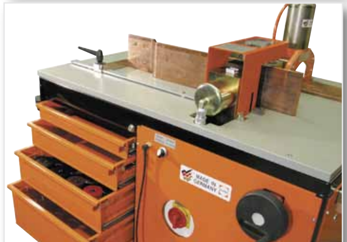
Inside the cart there are 4 tools drawers with compartments for punches and dies.
